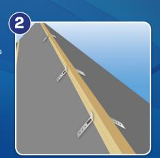
Using 30mm stainless steel annular ring shanked nails, fix a Batten Support Bracket to the apex of every rafter. Nail each bracket to the rafters through the holes on each side. Lay a batten between the support brackets and tile the roof as normal.
