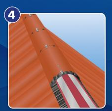
Lay the ridge tiles along the ridge, placing a Ridge Union between each pair of adjacent ridge tiles. Secure the ridge tiles to the ridge batten bu screwing the Clamping Plate over the ridge tile and into the ridge batten. After laying all the ridge tiles ensure the finishing ridge tiles are fixed at both ends. If mortar is not being used at the ends of the ridge, cap the ridges off with a block end ridge or ridge end cap.
