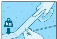
Use the self-adhesive Ready Roof Reinforcement Tape to cover all joints. laps, gaps and cracks, including any cuts you have made to the existing roof membrane whilst preparing the area.
