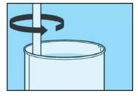
Thoroughly mix the Ready Roof liquid rubber using the paddle whisk provided on a low speed setting with your electric battery driver so as not to introduce air bubbles into the liquid.
