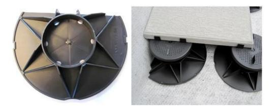
Contractors often ask how to pave up to the edges of upstands and walls when using adjustable supports. Because of the strength of the polypropylene support pads, the base plates can be cut with a saw to suit the shape of the edge upstand as shown above. The arms ensure that the weight is still evenly spread onto the base plate. Take care not to cut into the central core as this will lead to the support pad becoming unbalanced.
